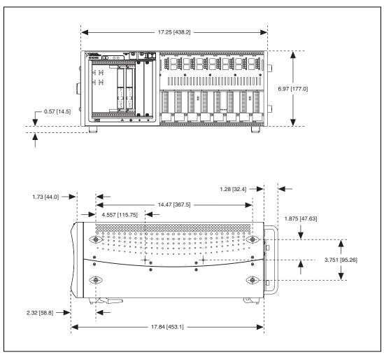
Figure A-1. PXI-1052 Dimensions (Front and Side) in Inches (mm)
